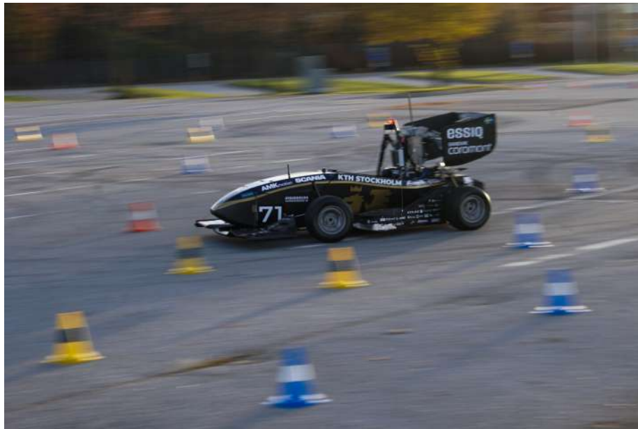
Figure 5: Dev18 driving autonomously during a testing session
