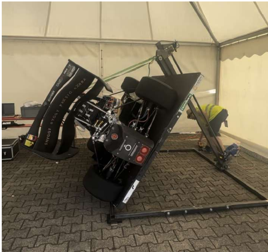
Figure 21: Dev18 in the tilt test
