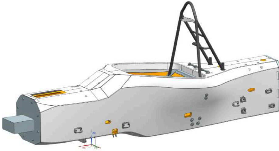
Figure 23: 3D model of the monocoque
